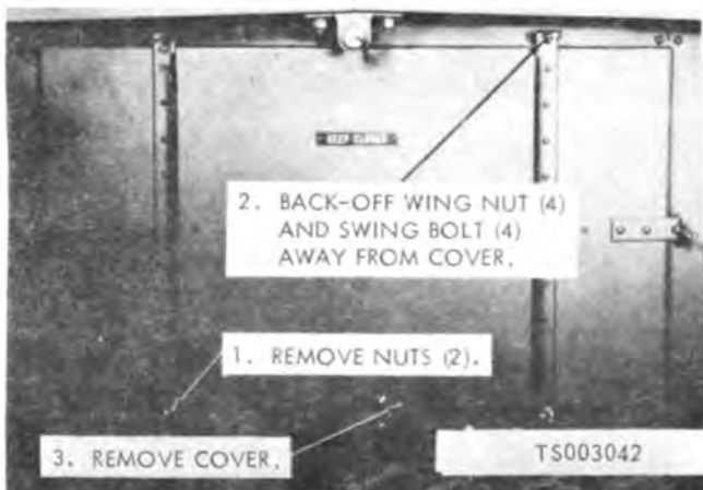
Figure 4-70. Bow hatch cover removal.
